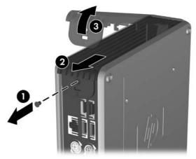
Figure 2-1 Removing the secure USB compartment cover
